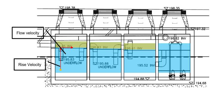
• All particles that rise up past the outlet pipe are captured before they pass out of the chamber.
